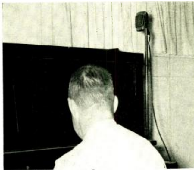
The best results from an upright or spinet can be had by moving the piano to a position at right angles to the wall or by placing it so the back faces the center of the room. If neither of these positions can be secured, open the top and place the microphone at the treble end of the keyboard. If possible, tilt the head downward toward the center of the strings. Mike should not touch the piano.
